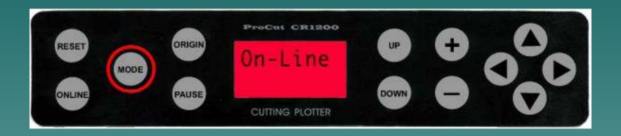
The plotter will go through a short memory test, then display 'On Line.'
