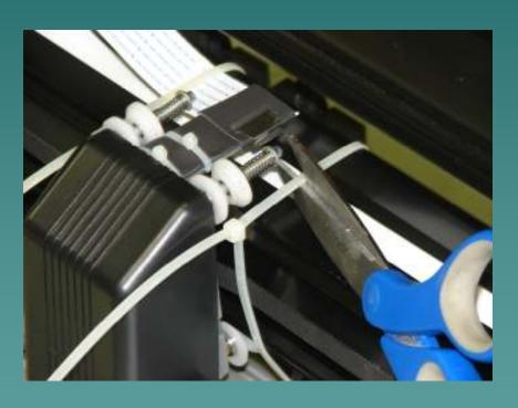
Brand new plotters will have 2 zip-ties (the longer zip-ties pictured here) holding the cutting head in place. Cut these out of the way, being careful not to cut the data cable.
