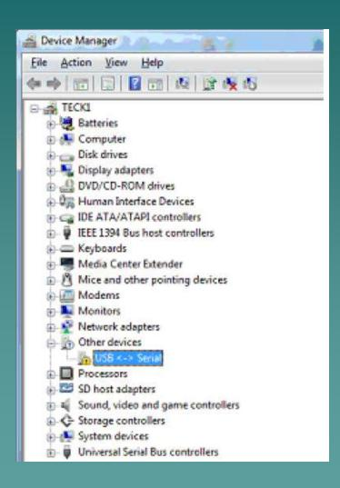
Scroll down and locate the USB<-> Serial device.
