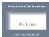
4.2.1.4 When the initializing is over, the machine is in online state and connectable with the computer to be operable.
