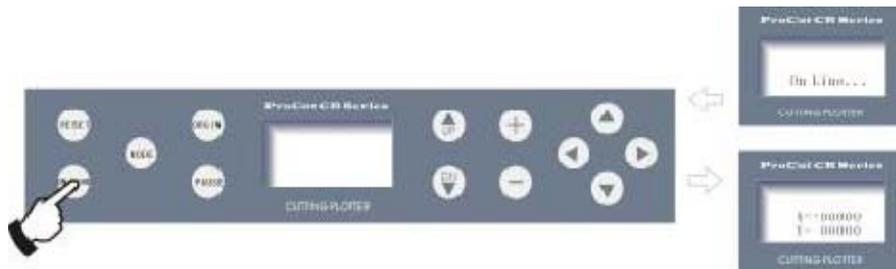
4.2.3.2 While in “off-line” state, press “ ” twice, the machine will automatically cut a small square from the media.
