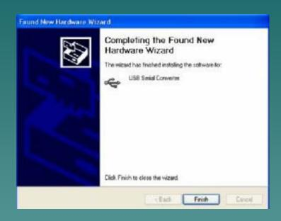
If the installation finished as "USB Serial Converter", the installation will need to be run once more. The end result when complete should read "USB Serial Port".
