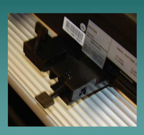
Loosen the tension on the pinch rollers by pushing the levers down.
