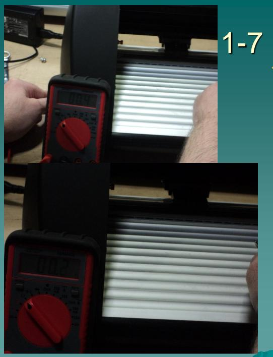
With the tips of the aluminum lightly sanded we can achieve a resistance to ground of only .2 ohms which is adequate to dissipate the vinyl static safely to ground.
