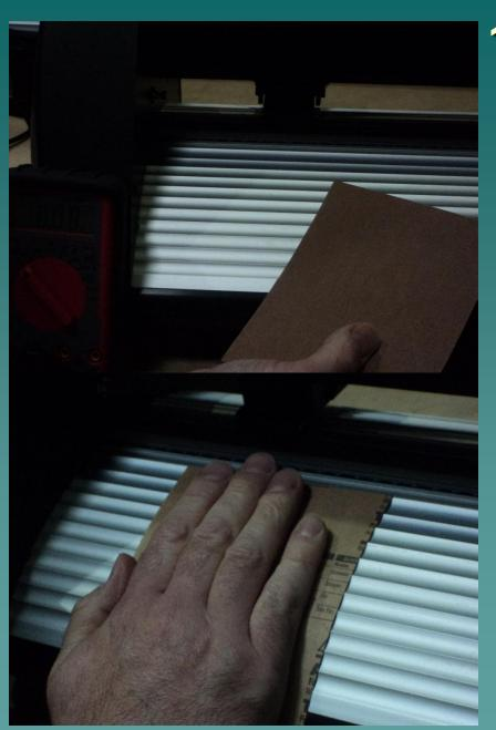
A light grit sand paper or emery board is used to remove the coating from the tips of the aluminum peaks where the vinyl rubs and comes into contact with the plate. Do this on both the front and back aluminum plates.
