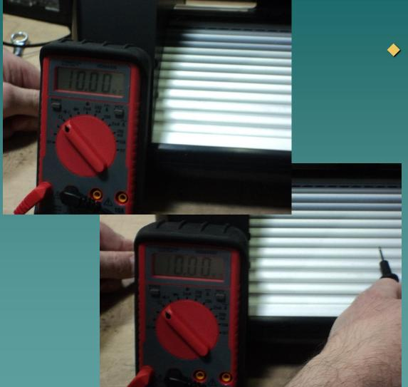
For CR series cutters, note that the resistance from the aluminum base plates to the ground plug is very high. The reason for this is due to a nonconductive clearcoat on the aluminum.
