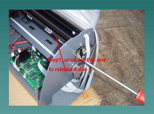
Loosen this screw to loosen the cable that guides the carriage.
