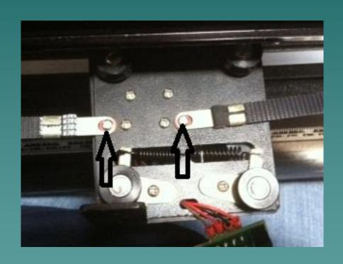
Loosen the screws on the back of the carriage to remove the cable.
