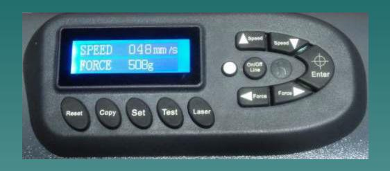
The cutter will go through a short memory test, then display the speed and force on the screen.
