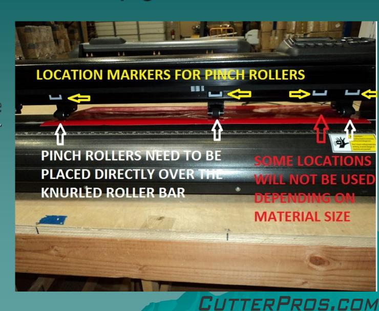
Note proper location of pinch roller. It is best to align pinch rollers prior to placing material in vinyl cutter.
