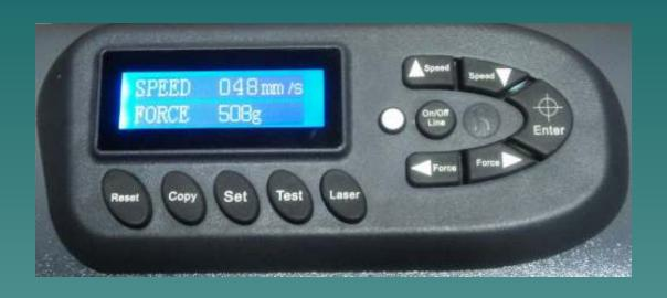
The plotter will go through a short memory test, then display the speed and force on the screen.
