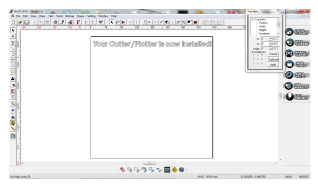
Select the Blue pen icon from the top toolbar to bring up the cutting panel; next change the Material width to match your substrate/Vinyl width and click on the design window to accept the new Material width configuration, select (Start) to begin cutting.
