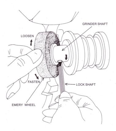
Hold the grinding wheel by hand. Insert the attached lock shaft to the hole provided in grinder shaft and turn to arrow indication. Remove used wheel and replace with new.
